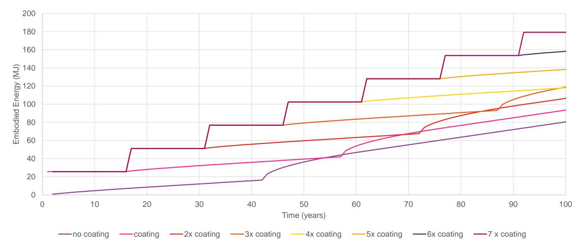
C3, 45 micron galvanised steel, steel = 35 MJ/kg
