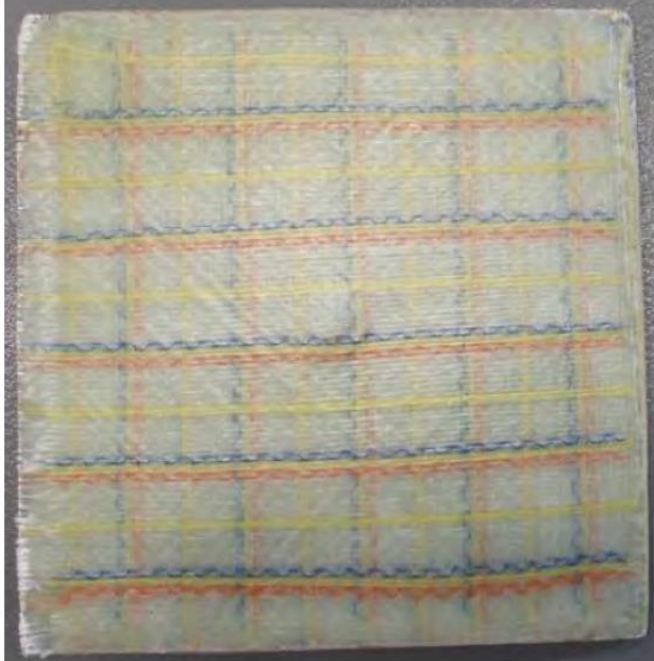
Composite repair on a flat plate
