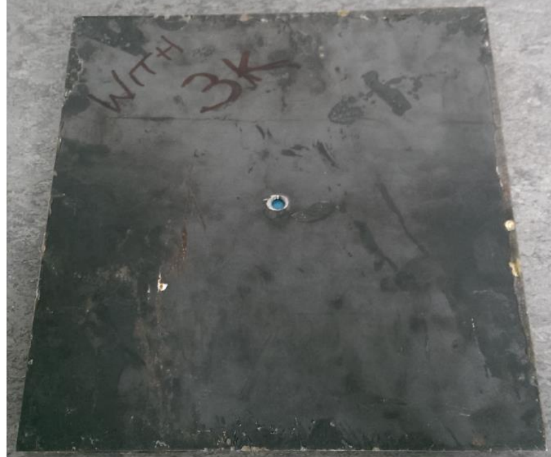
Pressure applied through back of plate to delaminate the composite
