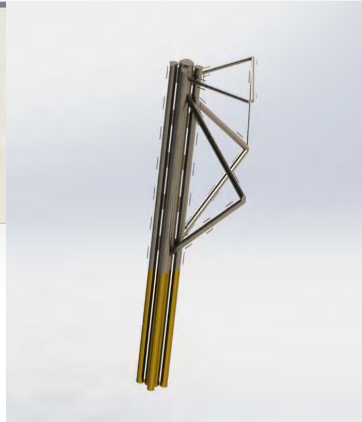
Local model of jacket section. Yellow section is mud zone. Galvanic anodes distributed on members.
