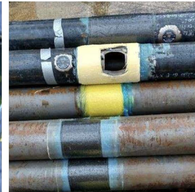
Pipe samples following pressure testing.
