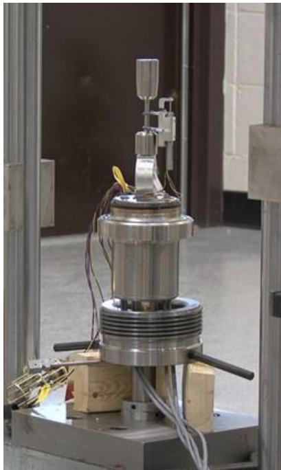
NIST High Pressure H2 Test Chamber - https://www.nist.gov/image/materialtestinghighpressurehydrogentestchamberjpg
