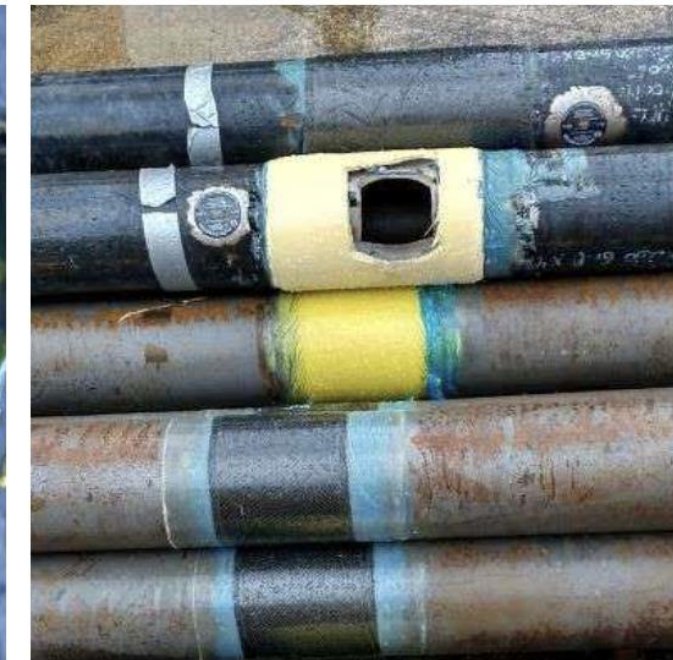
Pipe samples following pressure testing.
