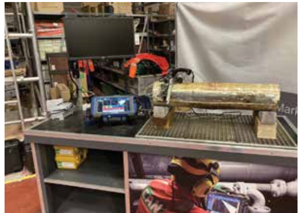
Photo: PA-CAT Tool (With Coating Stripped for Inspection).
