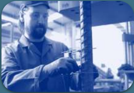
Testing of steel products for structural concrete
