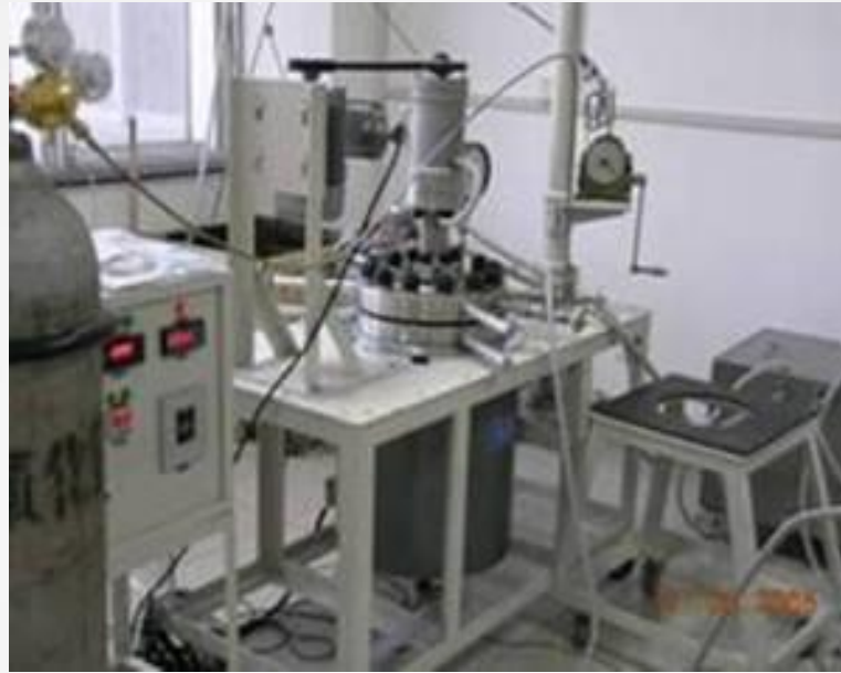
Autoclave (Dalian, China, 15 Sets) 30MPa/250°C/H 2 S/CO 2 /3m/s
