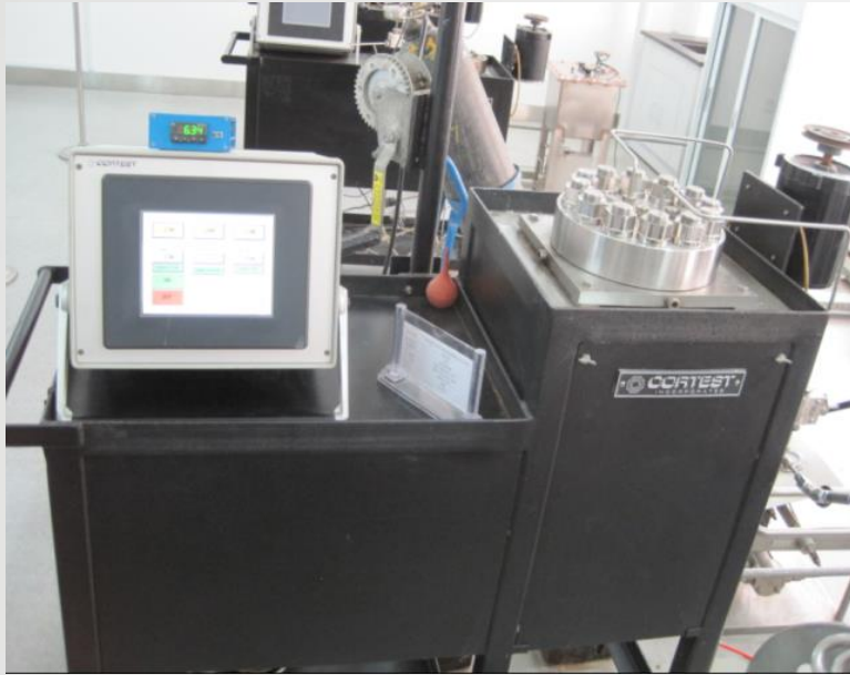
Autoclave Cortest, USA, 5 Sets) 70MPa/350°C/H 2 S/CO 2 /5m/s
