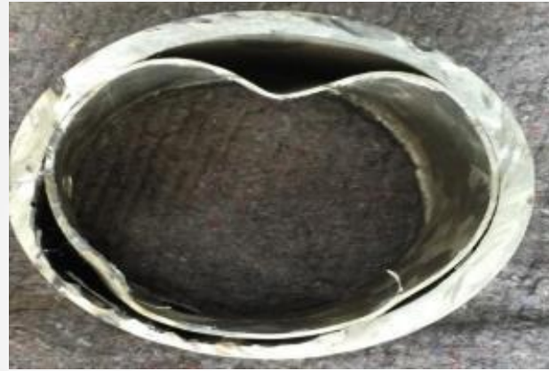
衬管塌陷 Liner Collapse
