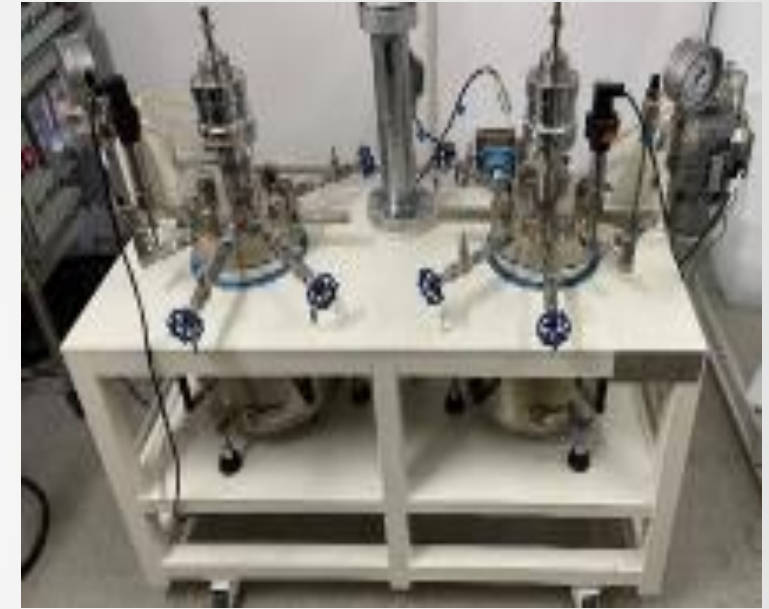
Twined-Autoclave (Dalian, China, 1 Set) 30MPa/250°C/H 2 S/CO 2 /3m/s
