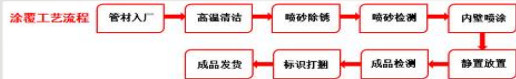
Coating Spray Process in Factory
