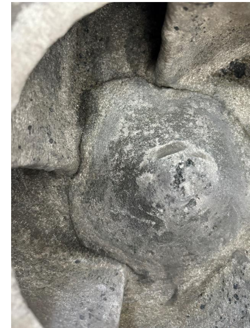
Corrosion cracking of impeller of poor amine solution transfer pump in CO 2 capture system
