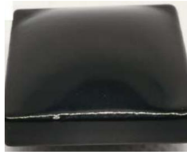
Blistering of the coating was observed under a high-pressure environment at 110 °C (Sun, et al. Surface Technology 51 (2022) 43–52)
