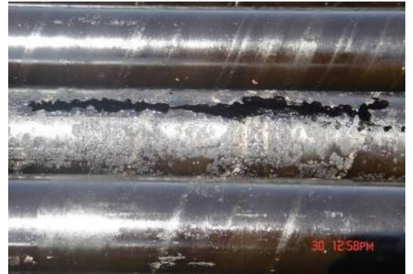
Downhole tubing corrosion failure
