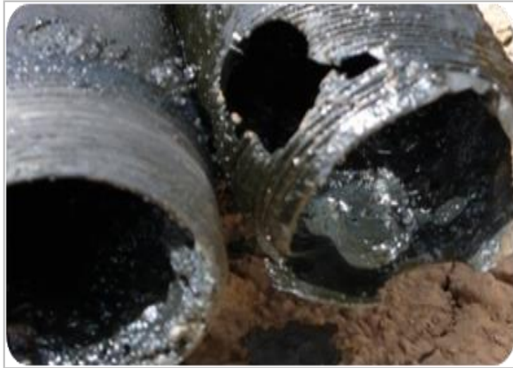
CO 2 -EOR well corrosion
